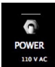
2 To begin, turn on the Power switch by clicking on it once. You will notice the left running light will glow red, indicating power, the Start Button will be illuminated, and the CRT-Style display will begin to warm up. After a few seconds the Display will show an empty graph (below, 3). The application is now ready to run a simulation.
